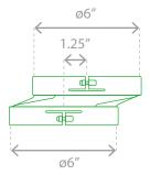
Air duct offset adapter included (inside dimensions)
